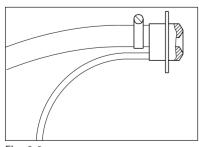
For smaller outputs of up to 4 kg/h steam, we offer a nozzle which can be either fitted in air ducts, for instance, or used for direct room humidification. The rules for vaporisation lines (lines needed to mix the steam adequately with air) must be observed here too.
